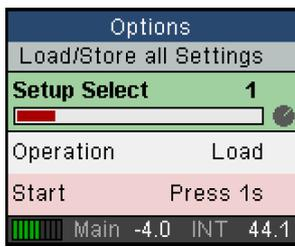
The Fireface UCX II can store and load its current state in 6 different memory slots, called Setups (SETUP/REV, Options, Load/Store all Settings). With this, the Fireface UCX II can be used stand-alone after setting it up accordingly, replacing lots of dedicated devices (see chapter 24).
