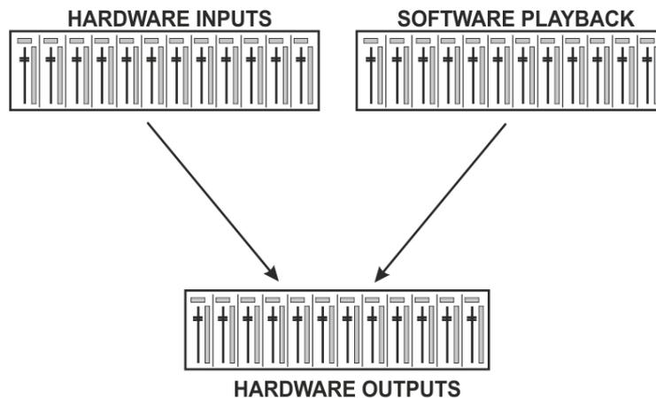
TotalMix can be used in the above view (View Options **2 Rows**). However, the default is a vertical alignment in three rows as known from an Inline desk, so that the row *Software Playback* equals the *Tape Return* of a real mixing desk:
