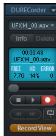
**Record View.** Switches from Mixer View to Record View. In Record View Mute and Solo buttons in first and third row are replaced by Play and Record (Arm) buttons.
