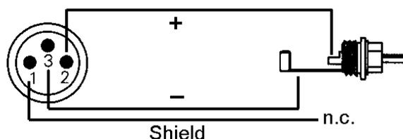
Using the cable adapter XLR/RCA described above, devices with coaxial SPDIF interface can be connected to the AES output of the Fireface UCX II as well. Note that most consumer equipment with phono (SPDIF) inputs will only accept signals having a Channel Status *Consumer*. In such cases the above adapter cable will not work.
