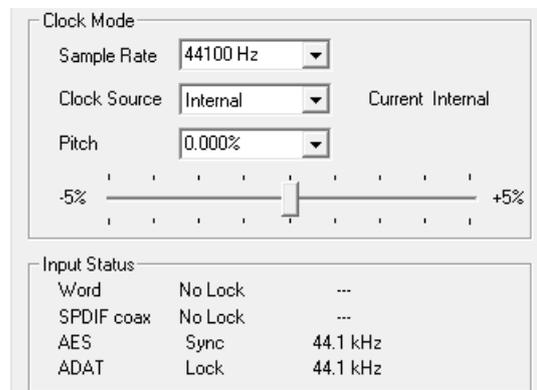
This way, configuring any suitable audio application for digital recording is simple. After selecting the correct input, Fireface UCX II displays the current sample frequency. This parameter can then be changed in the application's audio attributes (or similar) dialog.
