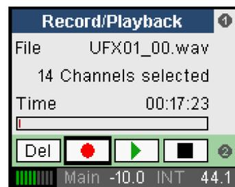
**Transport Bar.** Turning the encoder moves the cursor over *Del* (Delete), *Record*, *Play/Pause* and *Stop*. The selected function is initiated by pressing the encoder. During playback the buttons Del / Record will change to Previous File / Next File.
