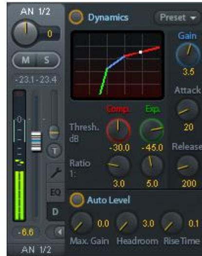
The amplitude graphics give a precise overview of the level changes caused by the current settings of Compressor and Expander. The white dot shows the level of the input signal and with this whether the signal is within the processing range or not. The small light blue lines in the level meter show the currently active gain reduction. Settings for these *Dynamic Meters* are found in the Preferences dialog (F2).
