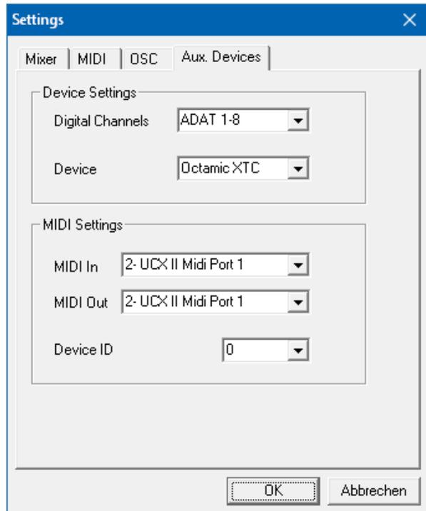
When using more than one OctaMic XTC these must have different Device IDs (configuration is done at the OctaMic XTC). *Aux Devices* supports to set different Device IDs to the 8-channel blocks as well. Storing the setting is done automatically when selecting a Device ID. To check the current assignments toggle the two 8-channel blocks.
