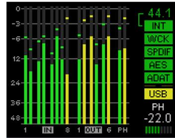
Turning the knob displays the volume screen of the currently selected output. Pressing the knob toggles the display between *Main Out* and *Phones*. At the bottom right, the current selection and dB value of the Volume setting is shown, so it is visible even when the Volume screen is not active.
