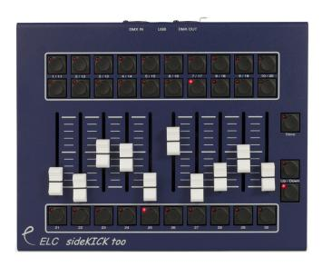
The sideKICK too provides a simple to use DMX scene capture and playback of 30 memories, each of which can be a single lighting state (up to 512 channels) or a chaser with individual period and crossfade times.
