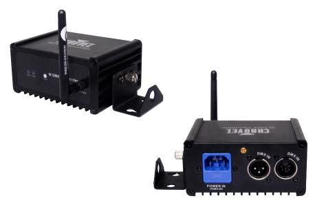
W-DMX<sup>™</sup> Transmitter works with W-DMX<sup>™</sup> wireless wash lights, including WELL<sup>™</sup> 2.0, to generate a wireless control signal. It features auto-ranging power from 100 to 240V, a locking IEC power connector and 3- and 5-pin DMX input-only connectors.
